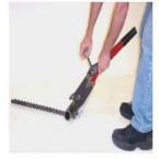
1. Place pipe on outstretched chain next to cutter jaws. Turn hand wheel counterclockwise until jaws are fully open.
