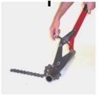
3. Rotate hand wheel clockwise to remove slack from chain.
