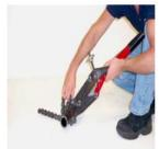
2. Wrap chain around pipe and engage nearest pin in upper iaw hooks.
