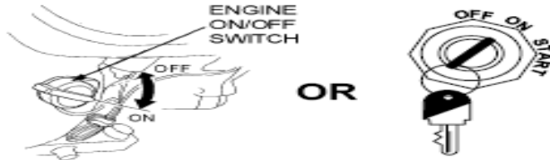
Figure 13. Engine ON/OFF Switch (Recoil Start)
