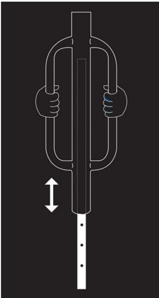
This is a simple tool, that is used to manually drive many different types of fence posts. From “T” posts, “U” posts, or any other type – as long as it fits inside the tube of the post driver.
